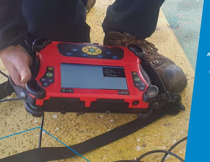
ACFM (Alternating Current Field Measurement) is an NDT technique used to detect and size surface breaking defect on both carbon steel and non ferromagnetic materials.
