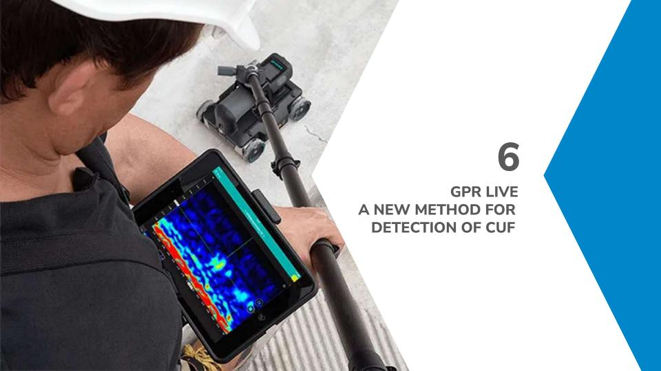
Ground Penetrating Radar (GPR) is a standard technique used for several scopes (mainly for structural inspection, locating rebar, 2D and 3D rebar layout reconstruction, etc.).
